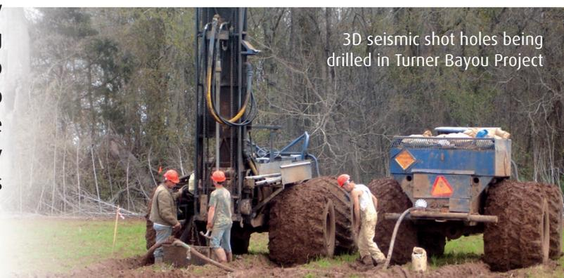
3D seismic shot holes being drilled in Turner Bayou Project
