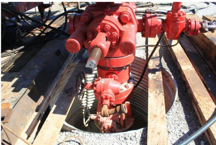
**Well head stack and blow out preventers (top left) Well head cellar and connection to casing (bottom left)
