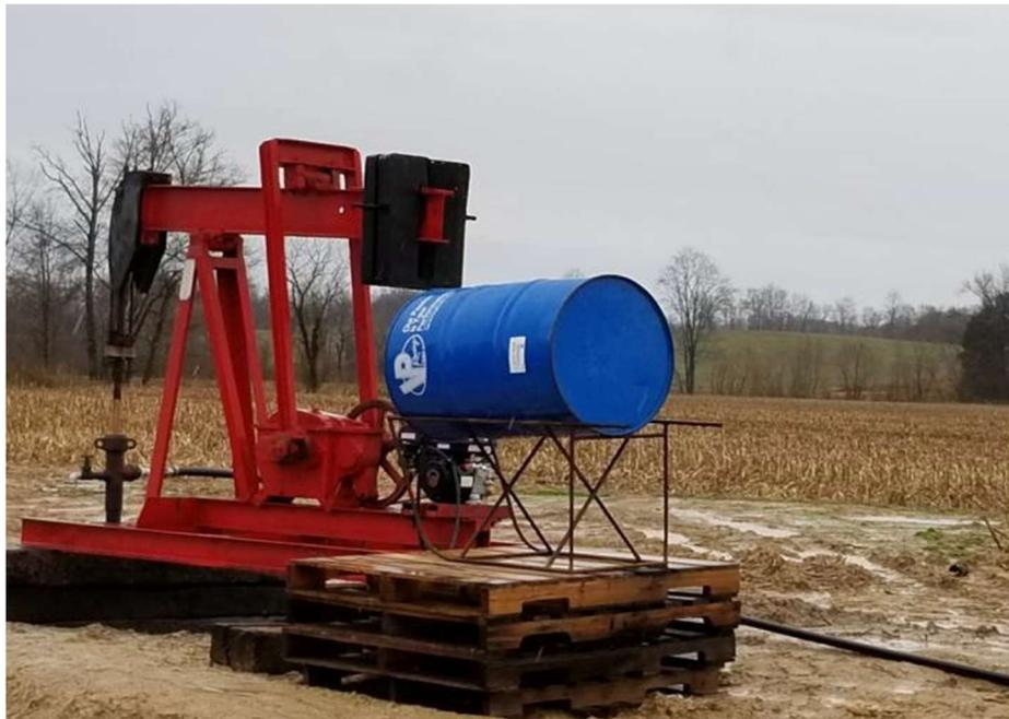
Figure 1. Recently installed pump on the Weldon Young # 1A well.
